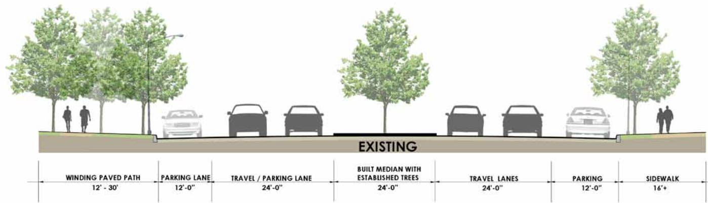
Riverdale Avenue Between Culver Street & Morris Street
